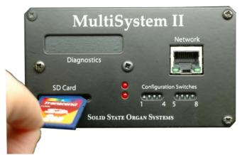
The CFMII uses a similar system to the MultiSystem II processors for the rest of the organ. However, in this case the SD memory card is always fitted and is used to store all the piston settings. There may be times when the card needs to be removed to update the system software. This card is labelled "Pistons" by the factory and needs to be back in the system before powering up to use the organ.
