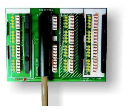
Pinboards have three wiring zones.
