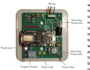
The Flip communicates wirelessly and so location is important to make sure the console parts do not interfere with the signal. Metal such as stop-jamb wiring will block the signal and thick wood will weaken it and possibly make the page turning unreliable. It may be a good idea to temporarily wire the Flip and test it in different
