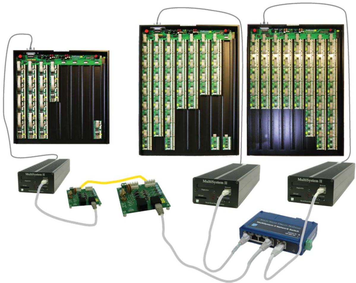
Figure 14: An example of a three location system
