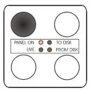
3/. Once the PANEL ON lamp is lit, push the LIVE button and hold in for three seconds until the disk can be heard being activated in the disk drive.
