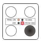
When the back up is complete the lamp will remain lit continuously for a short while and then go out. When the restore is completed simply push any general piston to reset the console.
