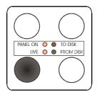
4/. When the LIVE lamp remains on with a steady glow the LIVE function is active and ready to use. Any pistons now set at the console within levels 1 to 32 will be recorded into Total Recall memory (not into the main MultiLevel Capture System memory).
