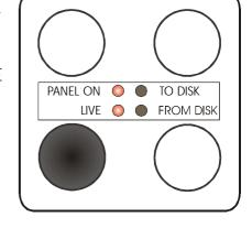
time but keeps them in its own memory until the LIVE button is pressed once more to exit. At this time, all registration settings within memory levels 1 to 32 are saved onto the disk. DO NOT remove the disk until the green light is off.
