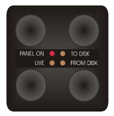
The complete Total Recall function is turned on and off using the PANEL ON button (top left). When the PANEL ON lamp is lit the other three buttons on the rest of the panel are operational.
